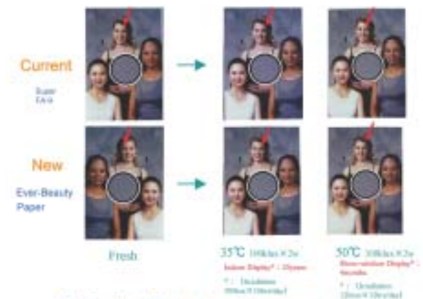
Fig. 3 Comparison of EVER-BEAUTY PAPER with the current paper on image permanence (effects of storage temperature).
