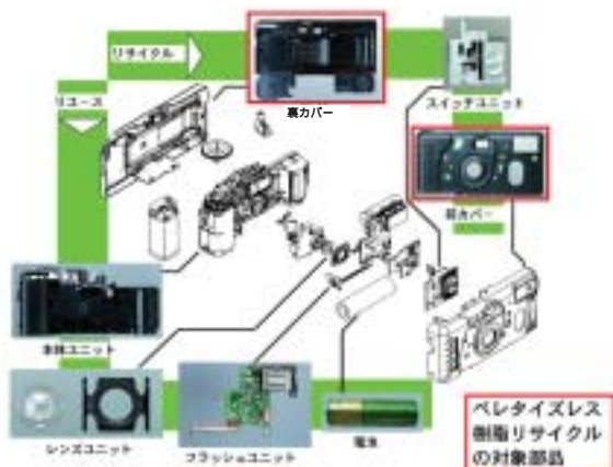
Fig. 2 Components of "Quick Snap".
