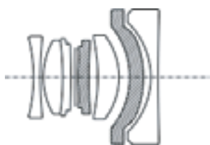
Fig. 8 Lens configuration of NATURA S (Slashed parts represent aspherical lens).
