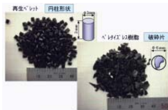
Fig.8 Difference in the shape of the plastic pieces used for molding.
