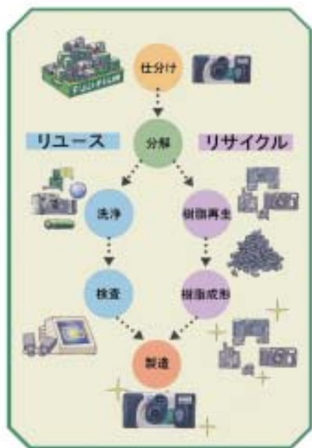
Fig. 1 Closed loop recycling.
