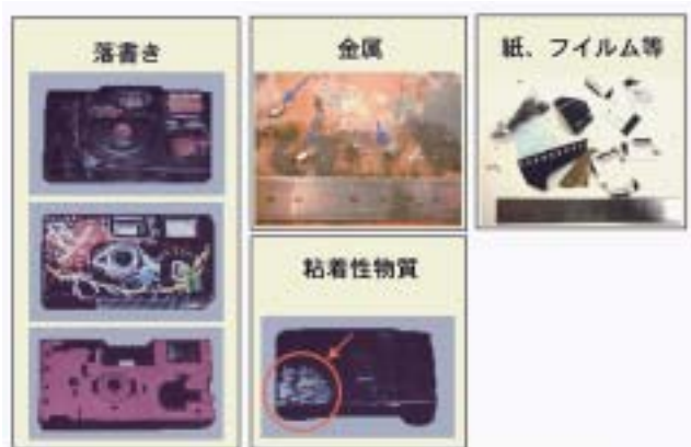
Fig. 9 Examples of the contaminations in used "Quick Snap".
