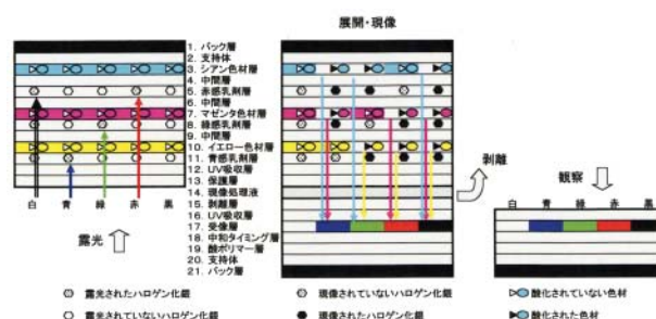
Fig. 1 Schematic sections of an instant film during exposure (left), processing (center) and viewing (right).
