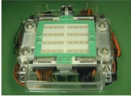
Fig. 6 Newly developed LED light source for film scanner.
