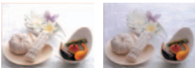
Photo 3 Photographs taken by FinePix S3PRO (left : using only S-pixel, right : using both of S-pixel and R-pixel).
