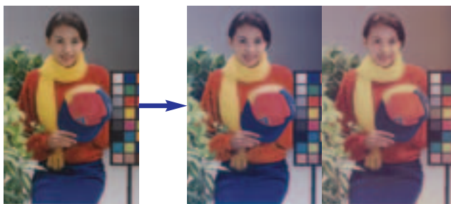
Fig. 8 Comparison of the new and current paper under ozone or NO 2 gas exposure.
