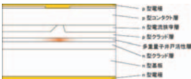
Fig. 2 Typical structure of a 660 nm band laser diode.
