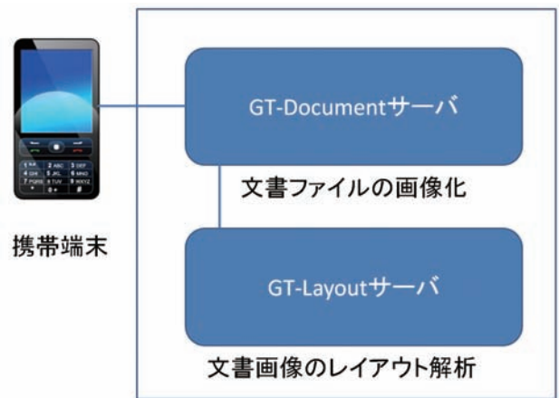
Fig. 3 System configuration of GT-Layout.
