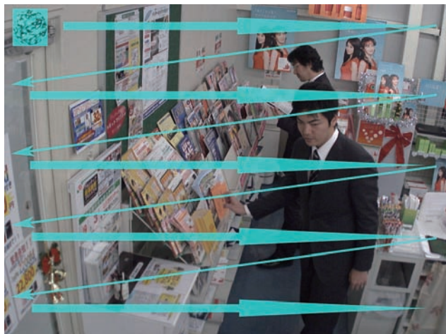
Fig. 6 Scanning procedure for head detection.
