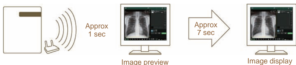
Fig. 7 FDR D-EVO plus C24i/s exposure cycle time.
